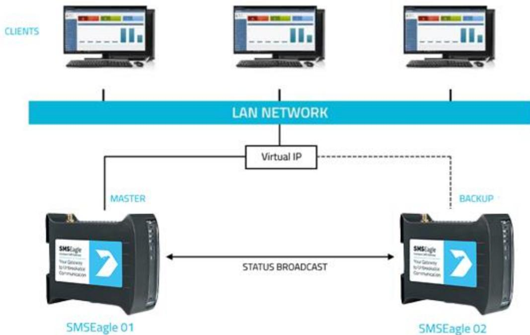
In the cluster you have one MASTER device and one BACKUP device. **HA-cluster is accessed via Virtual IP address.** When the daemon running at MASTER device detects failure of at least one described feature it immediately automatically switches cluster's IP assignment to the BACKUP device (node) providing continuous usage of the SMSEagle HA-cluster for the user.
