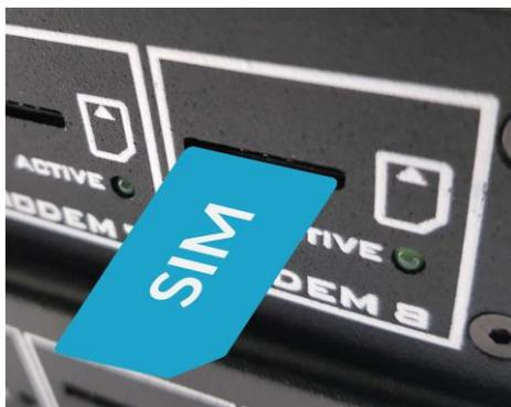
**Please install SIM Card when the device is SWITCHED OFF.** SIM Card slots is located on the front panel of the device. SIM metal contacts should face down when inserting SIM into slot.
