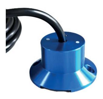
The industrial grade water leak sensor detects and alerts of a potential water leak emergency. When the water comes into contact with the sensor probe, it activates a relay that can trigger SMS alarm sent from SMSEagle device. The water leak sensor is designed with industry-standard IP66 rated, featuring waterproof and dustproof. The control circuit possesses minimal potential energy, mitigating the risk of igniting flammable or combustible substances.
